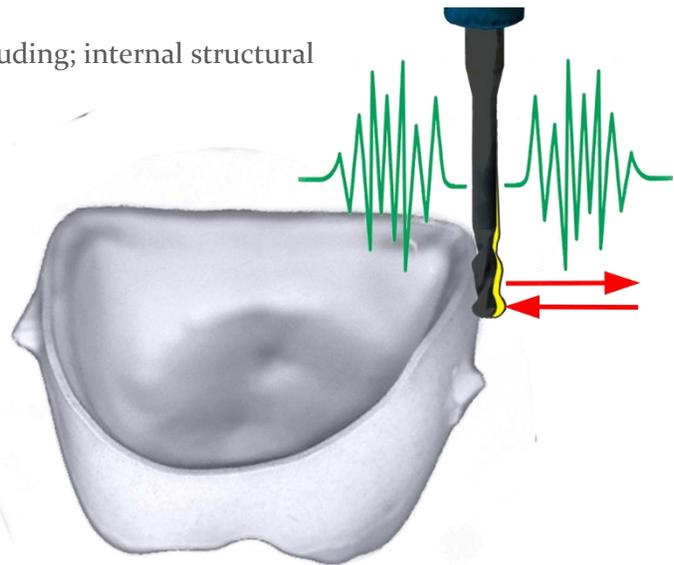
The structural integrity of the machine and fixture coupled with precision, high-torque spindles, robust CAM software and expert machining templates enable users to reliably produce high-quality restorations with clean, thin gingival margins and minimal margin reinforcement — as little as 40µm.
