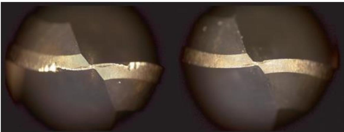
*Compare image of worn tool on the left with a new, unused tool on the right.*
