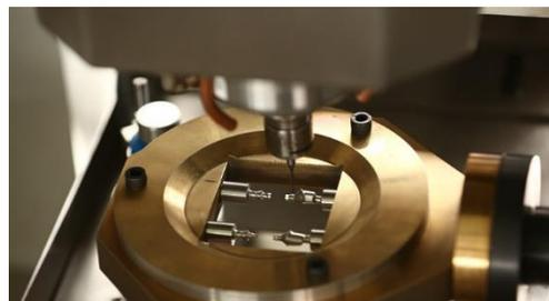
*Example of vibration inducing workholding: workpiece & fixture held on only one end.*
