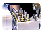
16-station ATC houses sturdy, flex-resisting 6mm diameter cutting tools with automatic tool management and breakage sensor.
