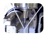
High-torque, .5kW max spindle with ceramic hybrid bearings that help to reduce margin thickness, and extend spindle life by reducing deflection and protecting against contamination by cutting chips and coolant.
