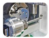
Precise assembly and testing of perpendicularity of A-axis and B-axis-vital for accurate multi-axis manufacturing.
