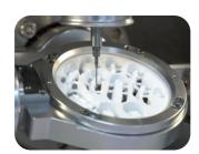
12-station ATC houses 3mm diameter cutting tools with automatic tool management and breakage sensor.
